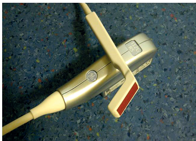
Fig. 2. Linear transducer (General Electric) adapted to the Vivid S6 device to perform ultrasonographic evaluation of the aorta and peripheral vessels
